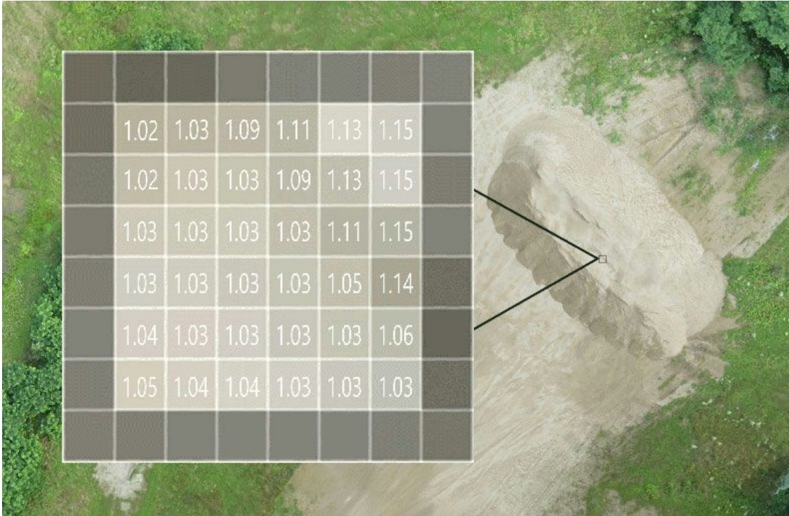
Illustration of relative pile elevations above estimated ground elevation for each point on the DEM
